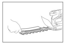
**NOTICE:** Do not wash the blades in water. Doing so may cause rust or damage to the tool.
