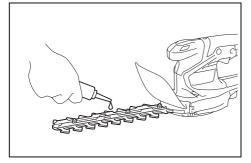
After operation, remove dust from both sides of the blades with a wired brush, wipe it off with a cloth and then apply low-viscosity oil (machine oil, or spray-type lubricating oil) to the blades.
