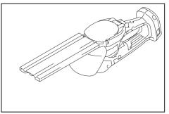
2. While pressing the lock lever, turn the undercover counterclockwise until  $\mathbf{a}^0$  on the undercover is aligned with  $\Delta$  on the lock lever.
