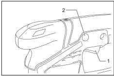
1. Switch trigger 2. Lock-off button
