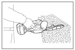
For basic operation, tilt the blades toward the trimming direction and move it calmly and slowly at the speed rate of 3 to 4 seconds per meter.
