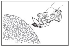
Trim large branches to the desired height using branch cutters before using this tool.
