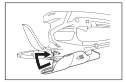
**NOTICE:** Do not attach the hinge of the grass receiver to the tool forcibly after aligning the protrusions on the grass receiver with the grooves on the tool.
