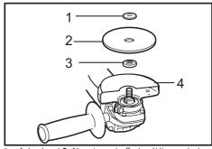
1. Lock nut 2. Abrasive cut-off wheel/diamond wheel
