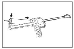
**3.** Push the rod gently until the piston touches the bottom of cartridge.
