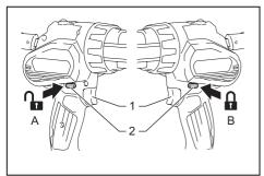
1. Switch trigger 2. Trigger-lock button
