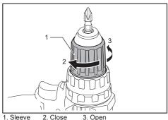
Turn the sleeve counterclockwise to open the chuck jaws. Place the driver bit/drill bit in the chuck as far as it will go. Turn the sleeve clockwise to tighten the chuck. To remove
