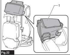
• 1. Protection cover (for the battery adapter)
