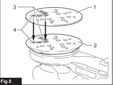
Pad saver 2. Pad 3. Screw holes 4. Dust-suction holes
