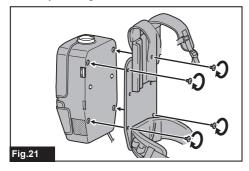
4. Store the battery parts of the battery adapter in the protection cover (for the battery adapter), and then loop the protection cover (for the battery adapter) on the harness as shown in the figure.
