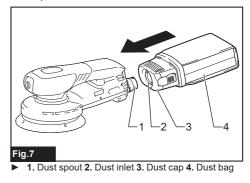
**NOTICE:** Do not hold the dust bag when carrying the tool. Otherwise, the tool may fall and be damaged.
